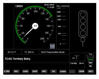
• After passing two RFID tags (for getting direction) and communication from stationary Kavach, the on board Kavach will automatically enter in to 'On sight' mode.
